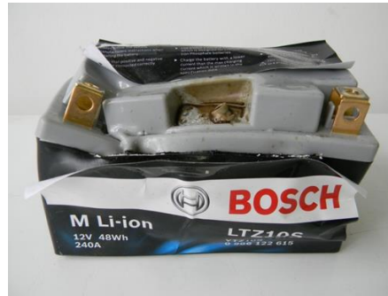
Image 6: Images tested battery / cell pack (after opening) after overcharging test
